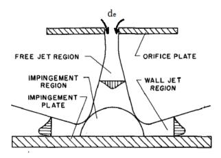
A common correlation for the heat transfer on a flat surface in the impingement region beneath an impinging air jet is
