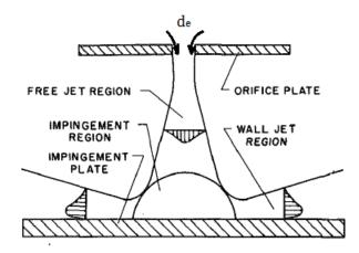
A common correlation for the heat transfer on the flat surface in the impingement region beneath an impinging jet is
