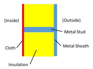
Draw a thermal resistance network for the different heat transfer pathways for this system. Clearly identify which pathways are in series and which are in parallel. Write an expression for the overall thermal resistance of the wall.
